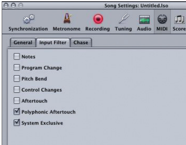
Fig. 4 : Logic's MIDI Input Filter song setting lets you filter out MIDI messages that you don't want recorded in your MIDI region.
