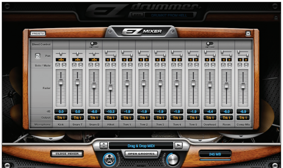
Fig. 2: The mixer. Note the Bleed control, which simulates the mic leakage that's such an important part of a recorded drum kit.
