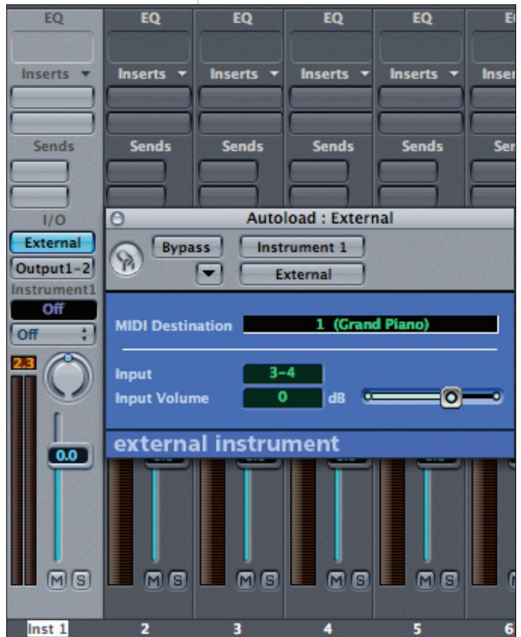
Fig. 5: Insert an External Instrument plug-in on an Instrument track to route external hardware instruments—or stand-alone V.I.s running outside Logic—into the mixer.
