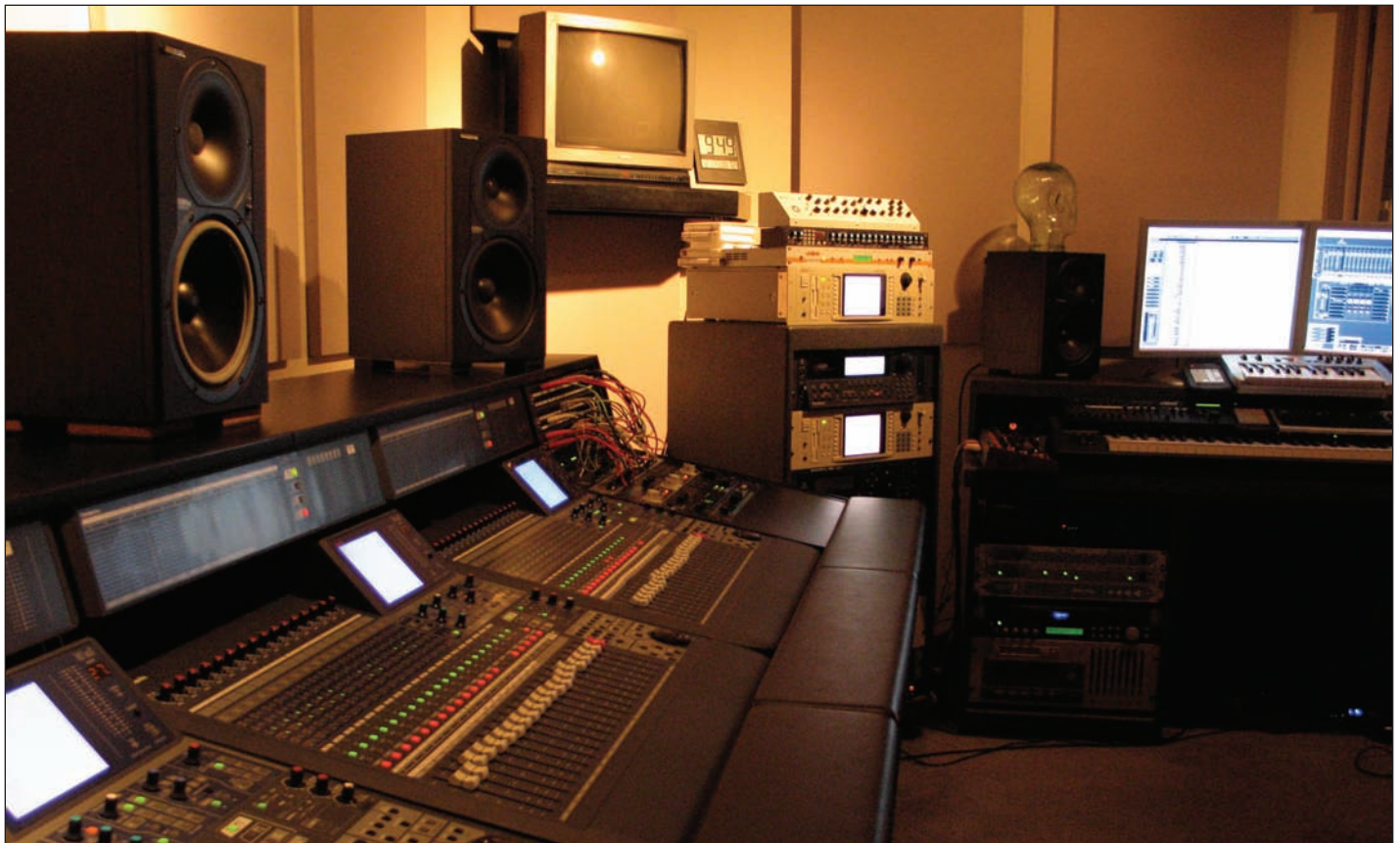
Fig. 3: Keresztes' studio is based around three (now discontinued) Panasonic DA7 digital mixers.
