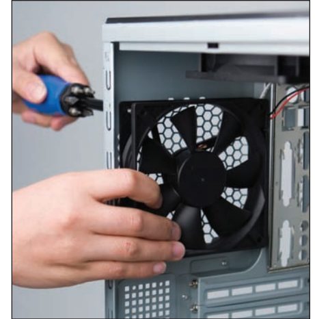
Fig 3. Typical fan installation in a case
