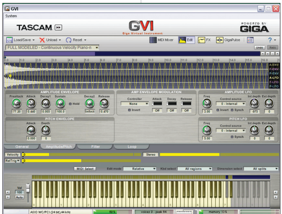
Fig. 3: As in its filter editing screen, GVI's amplitude/pitch envelope or LFO modulation is represented as a line superimposed over the waveform. This sine wave pattern here is a tremolo effect created by modulating the amplitude with an LFO.
