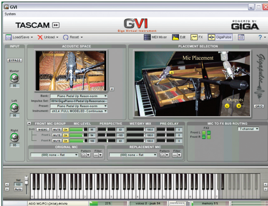
Fig. 2: The GigaPulse convolution processor is built into Giga GVI. Convolution isn't only for reverb—this program is TASCAM's continuous velocity piano, which is using convolution to model the pedal up resonance. Embedded convolution programming is a big part of Giga.
